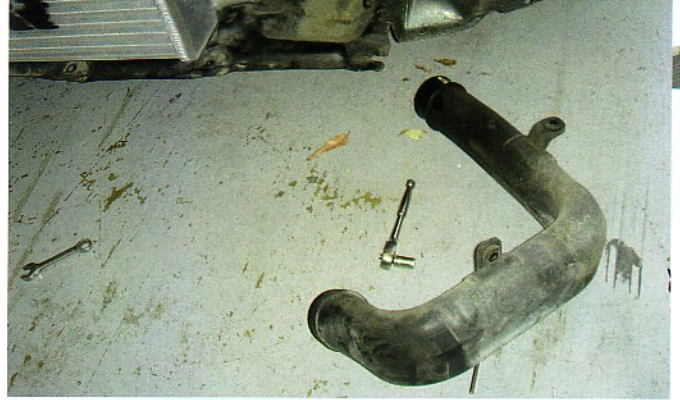
This plastic pipe normally runs through the space you see next to the intercooler outlet pipe
