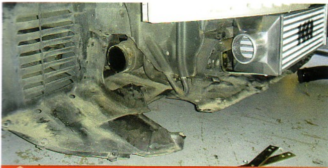
On the driver's side, it is a 180° bend around to the intercooler inlet
