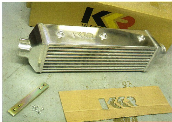
The KKR PI-1 core measures 520mm long, 160mm high and a fat 127mm thick. By comparison, the stock core is 210x270x98mm, or around half the overall volume
