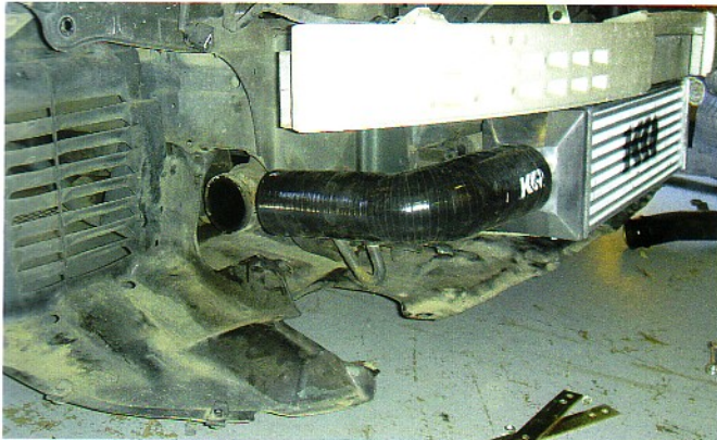
A KKR 90° bend takes care of the first part, also dropping down from the 3in intercooler inlet size to the 2.5in standard piping size
